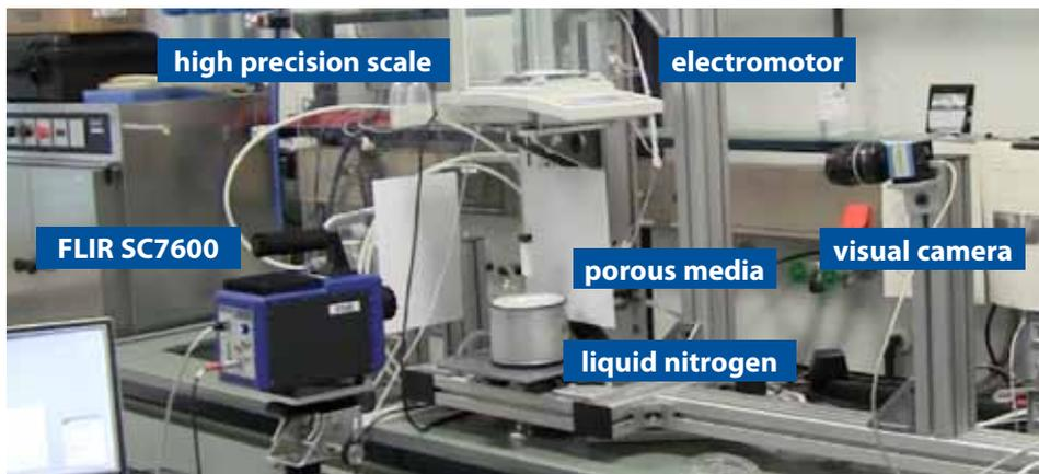
*In this test setup the electromotor is used to dip the porous media in the liquid nitrogen. The high precision scale measures the change in weight and the FLIR thermal imaging camera provides information about the speed with which the liquid nitrogen travels up the porous media.*
