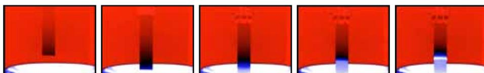
*This sequence of thermal images shows the wicking test result for the woven mesh made of stainless steel.*
