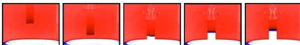
*This sequence of thermal images shows the wicking test result for the porous glass frit.*
